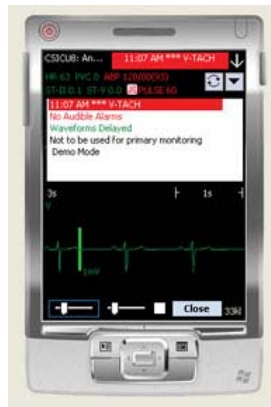
Philips' remote viewing capability displays moving waveforms on a PDA in near real-time.
