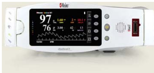
Masimo's Radical-7 Pulse CO-Oximeter featuring Masimo Rainbow SET can now be upgraded to include a continuous noninvasive total hemoglobin (SpHb) measurement.
